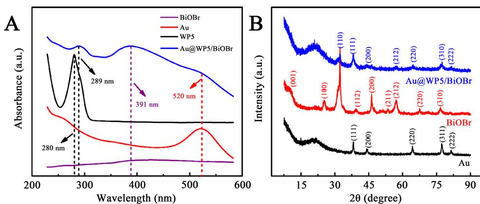
**Figure 2.** (A) Ultraviolet-visible diffuse reflectance spectra (UV-vis) of Au, WP5, BiOBr, Au@WP5/BiOBr; (B) The XRD patterns of Au@WP5/BiOBr
