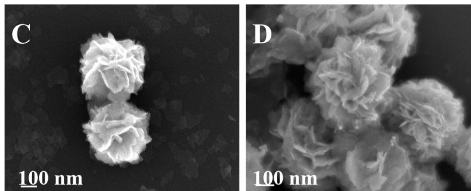
**Figure 1.** (A) (B) TEM images of AuNPs at different magnifications, (C) SEM images of BiOBr and (D) Au@WP5/BiOBr
