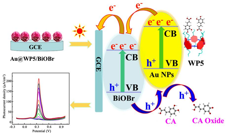
**Scheme 1.** Detection mechanism of the photoelectrochemical sensor
