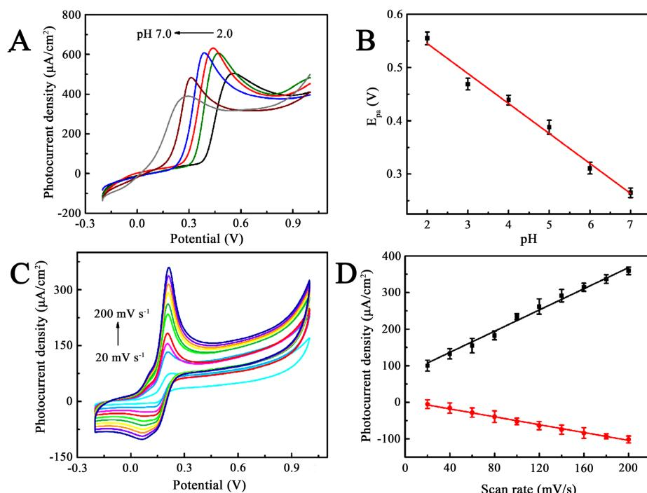
**Figure 4.** (A) The CVs of the Au@WP5/BiOBr/GCE in  $0.1 \text{ mol/L}$  PBS solution containing  $0.5 \text{ mM}$  caffeic acid under visible-light illumination at various pH values from 2 to 7; (B) Peak potential versus pH values; (C) CVs of scan rates from 20 to  $200 \text{ mV s}^{-1}$  in  $0.5 \text{ mM}$  caffeic acid; (D) The corresponding plots of anodic and cathode oxidation peak photocurrent densities versus the scan rates
