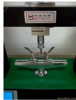
Figure 11. Three-point bending test 图 11. 三点折弯试验
