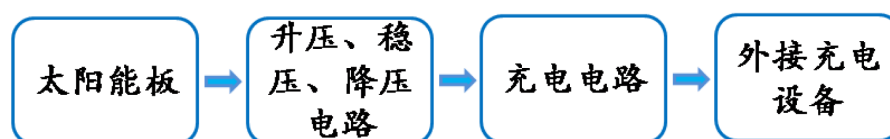
Figure 1. The principle structure diagram of solar charger.
