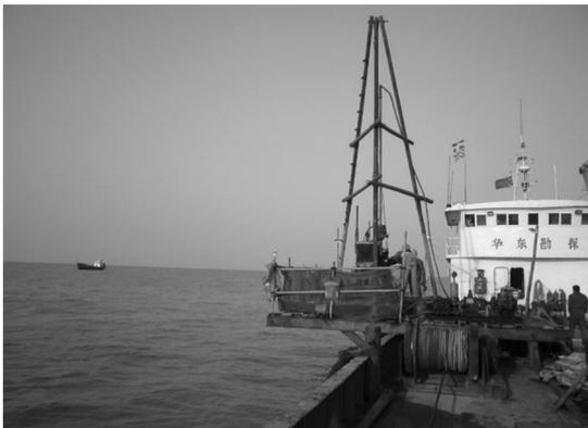
**Figure 1.** Single drilling vessel built on one side of the vessel
