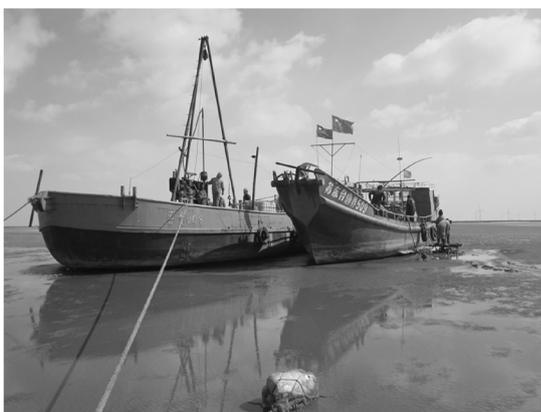
**Figure 2.** The single drilling vessel with reserved through hole
