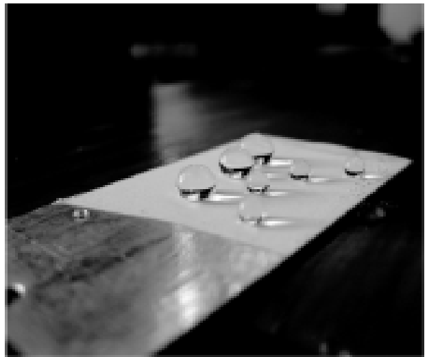
Figure 1. Water droplets' condition in coating surface [23] 图 1. 水滴在涂层表面状态 [23]
