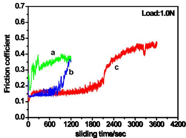
**Figure 5.** Friction coefficient as a function of sliding time when sliding a steel ball against (a) bare steel, (b) the NiO-TiO<sub>2</sub> film on steel and (c) the NiO-TiO<sub>2</sub> film after modified by stearic acid at load of 1.0 N
