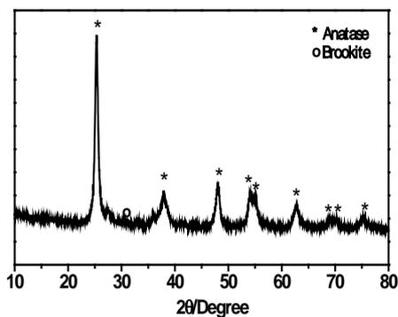
Figure 1. XRD analysis of NiO-TiO<sub>2</sub> powders
