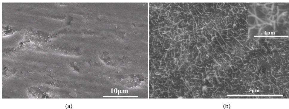
Figure 2. SEM image of (a) bare steel and (b) NiO-TiO<sub>2</sub> film on steel
