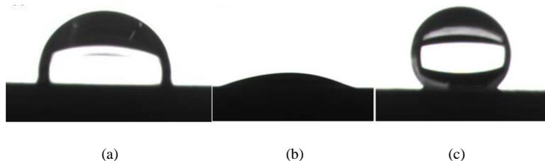
Figure 3. Water droplet images for (a) bare steel, (b) NiO-TiO<sub>2</sub> film on steel, and (c) NiO-TiO<sub>2</sub> film after chemical modified by stearic acid
