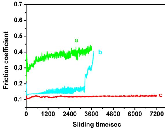
**Figure 4.** Friction coefficient as a function of sliding time when sliding a steel ball against (a) bare steel, (b) the NiO-TiO<sub>2</sub> film on steel and (c) the NiO-TiO<sub>2</sub> film after modified by stearic acid at load of 0.5 N
