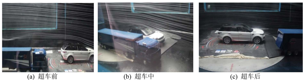
Figure 6. Flow field atlas of flue gas and wind tunnel experiments 图 6. 烟风洞实验流场图谱
