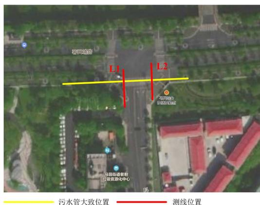
Figure 3. Layout of the field survey line of the transient electromagnetic method
