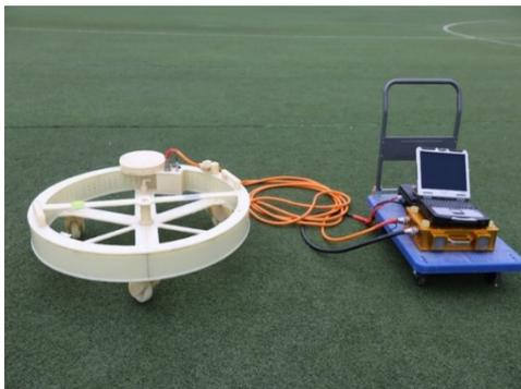
Figure 2. High-resolution towed transient electromagnetic detection system
