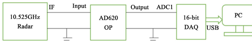
Figure 3. IF signal amplification and acquisition architecture 图 3. IF 信号放大与采集系统框图
