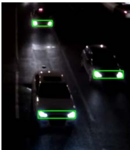
Figure 11. The result of headlight matching and vehicle detection 图 11. 车前灯匹配和车辆检测效果
