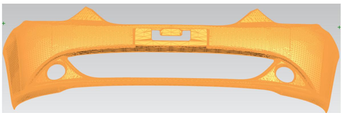
**Figure 6.** Triangular surface of the car's frontal
