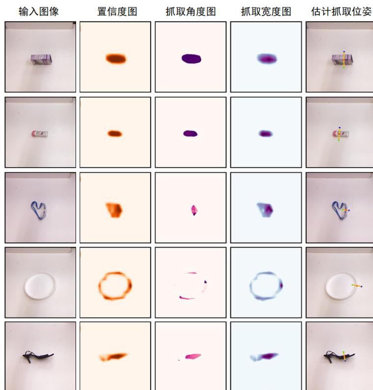
Figure 5. Visualization of grasp detection results on cornell dataset
