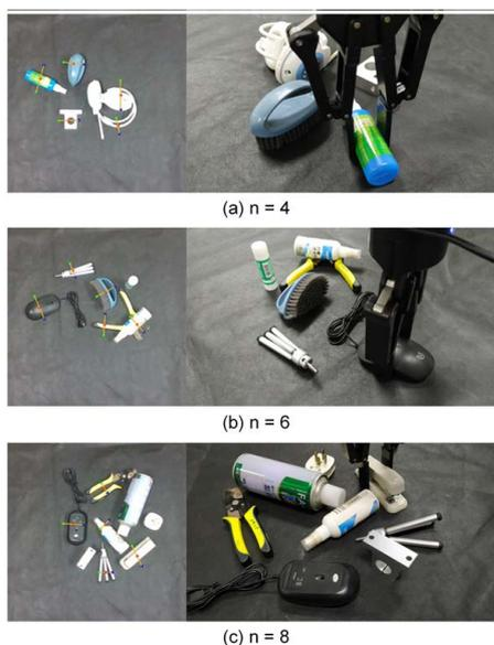
**Figure 8.** Illustration of robotic grasping in clutter scenarios
