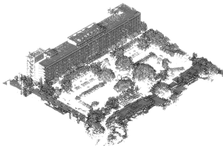
Figure 1. The results of morphological filtering (only retains ground object information) 图 1. 形态学滤波后的结果(结果仅保留地物信息)
