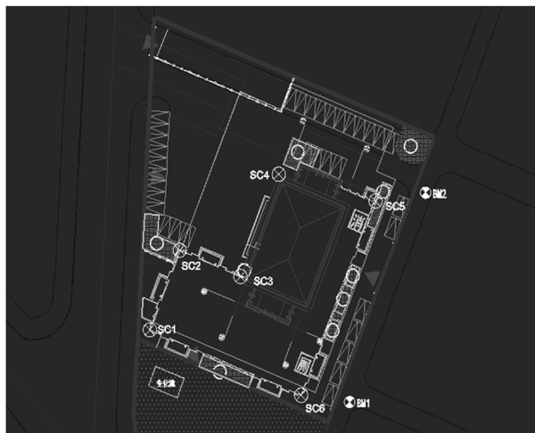
Figure 1. Plane layout of settlement monitoring points 图 1. 沉降监测点平面布置图
