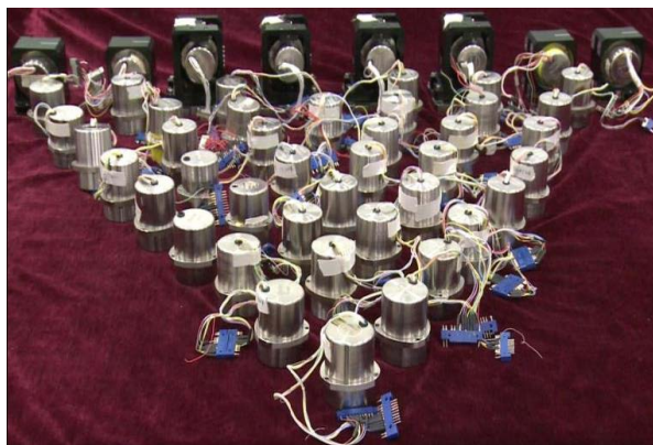
Figure 6. High resolution quartz flexible accelerometer [27]
