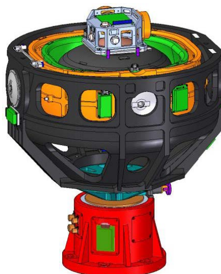
Figure 9. The stabilization platform of gravity gradiometer [22]
