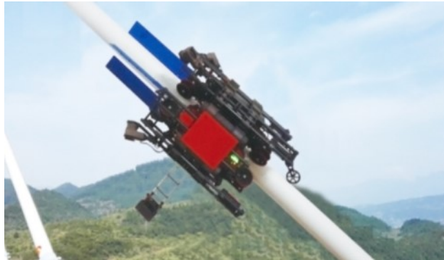
Figure 1. Diagram of cable detection robot 图 1. 缆索检测机器人图
