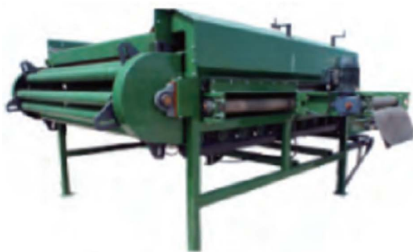
Figure 2. Roller potato grading machine
