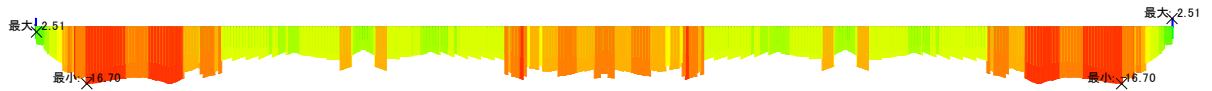
Figure 8. The maximum normal pressure of concrete under short-term condition 图 8. 短期状况下成桥混凝土法向最大应力图
