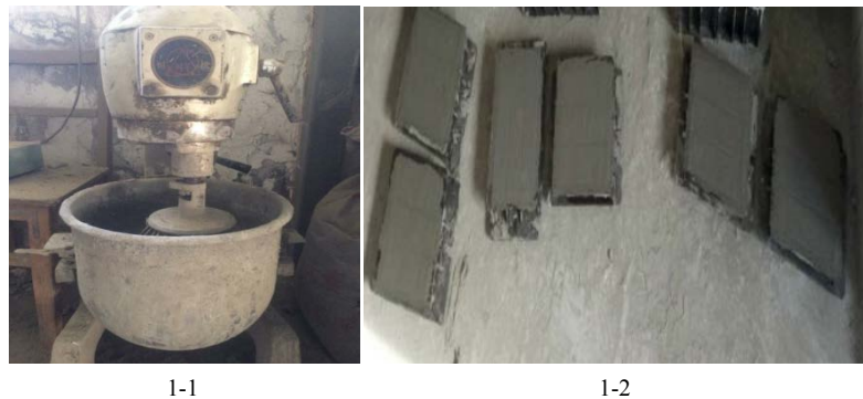
Figure 1. Test piece preparation 图 1. 试件制备
