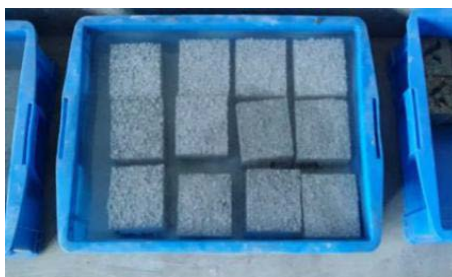
Figure 3. Curing of pervious concrete block 图 3. 透水混凝土试块的养护
