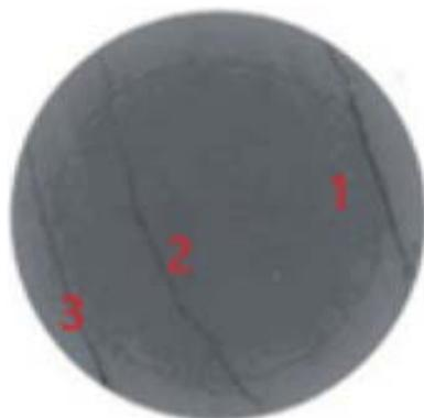
Figure 3. CT image of a core with cracks
