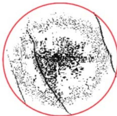
Figure 2. Shale binary image segmented by threshold method
