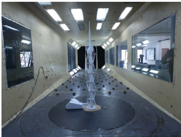
Figure 1. Wind tunnel pressure measurement model and turntable 图 1. 风洞测压模型和转盘
