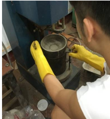
Figure 2. Compaction test 图 2. 击实试验
