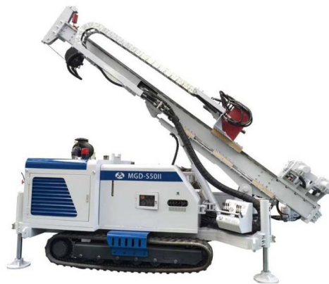
Figure 1. MGD-S50 II acoustic vibration drill 图 1. MGD-S50 II 型声频振动钻机
