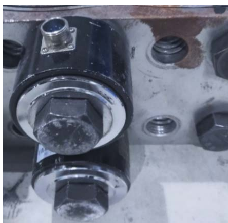
Figure 2. Installation diagram of through center pressure sensor
