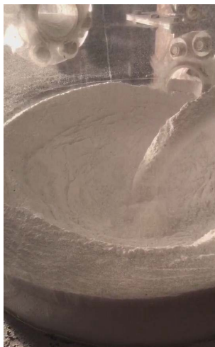
Figure 6. Solid flow way of the lateral discharges 图 6. 流化罐内料面下降实物照片
