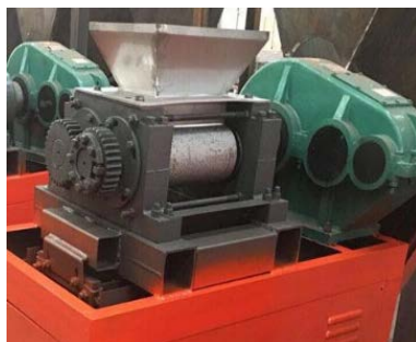
Figure 8. Twin rolling squeezing granulation 图 8. 对辊挤压造粒
