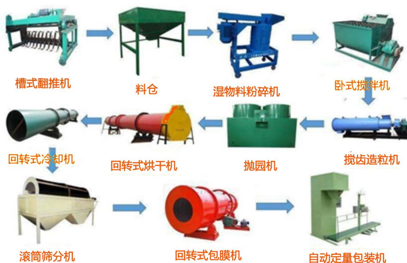
Figure 3. The overall system of organic fertilizer producing 图 3. 有机肥生产系统
