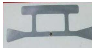
Figure 4. Ultra high frequency RFID hot stamping label in the paper substratum
