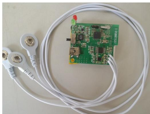
Figure 4. Picture of wireless ECG sensor node
