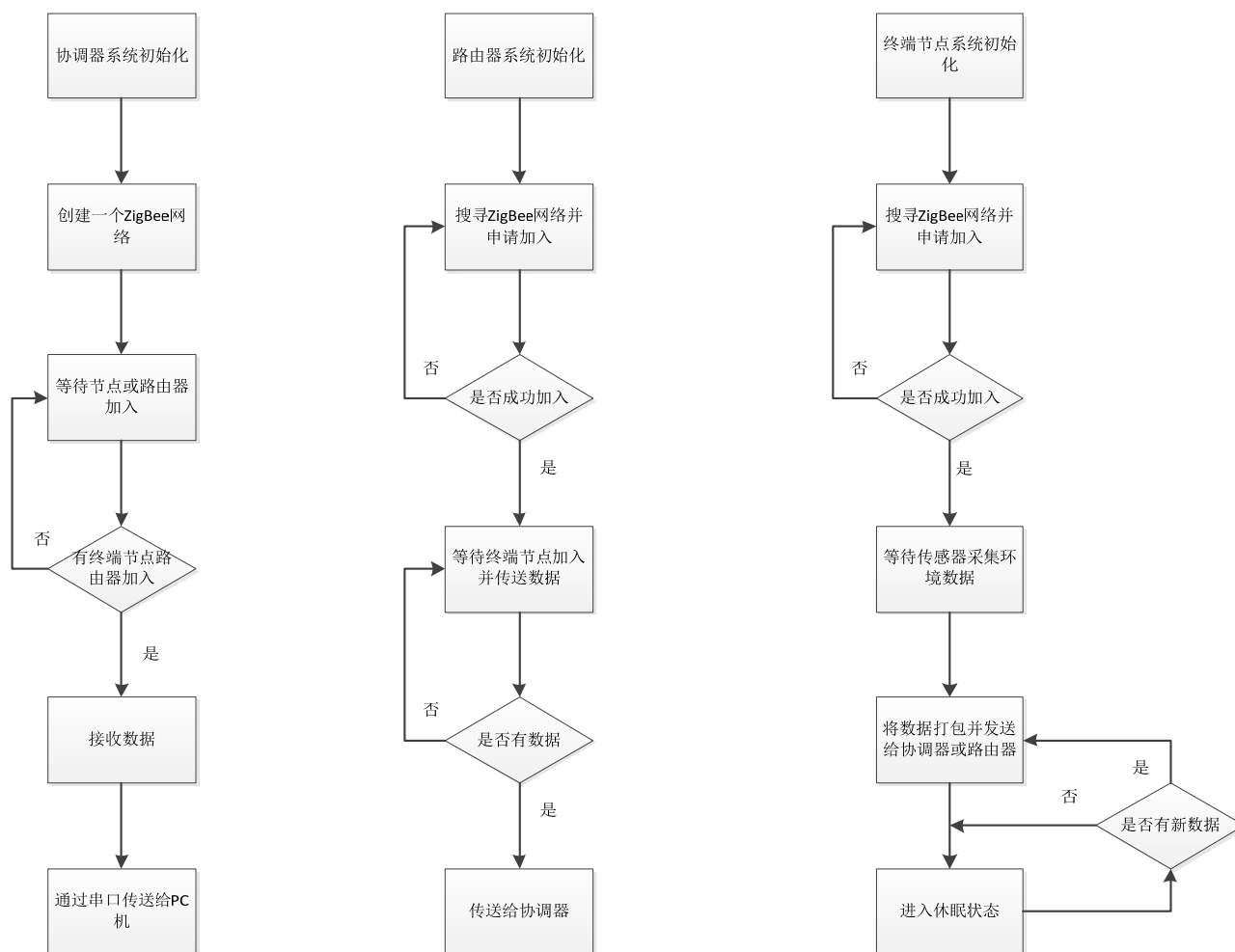
Figure 6. Boot workflow of zigbee 图 6. ZigBee 启动流程图
