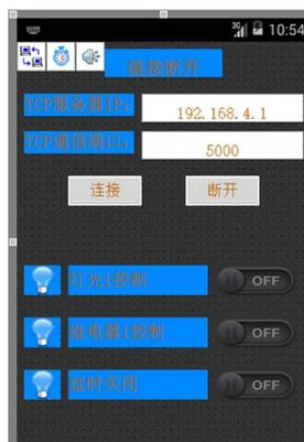
Figure 6. Control main interface design
