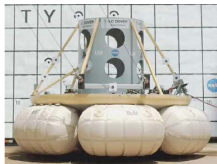
Figure 7. Airbag system installed on test article designed by NASA 图 7. 美国 NASA 设计的组合型气囊实验装置
