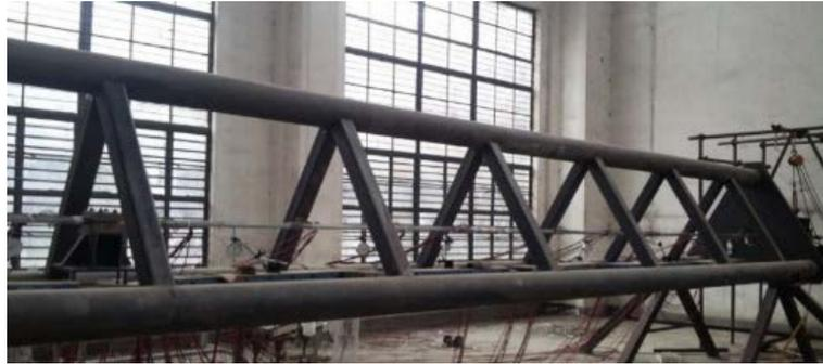
Figure 1. Self-balanced steel frame on model test site
