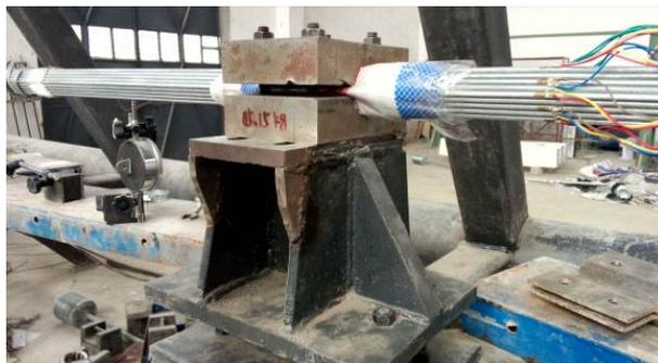
Figure 4. Temporary clamp on model test site
