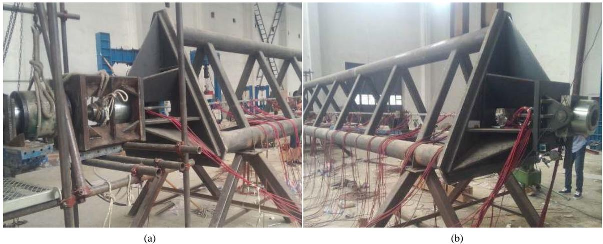
Figure 3. Loading on site of model test strands: (a) Strand axial force loading; (b) Strand end bending moment loading
