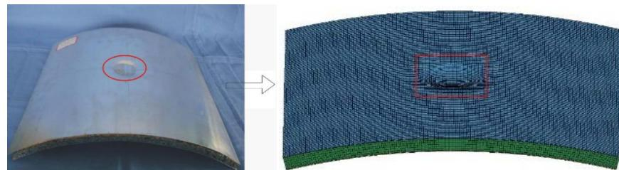
**Figure 4.** Deformation of aluminum foam sandwich shell
