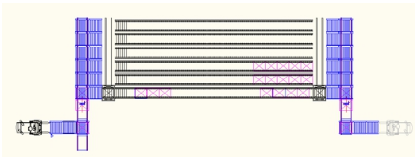
Figure 1. The plan of power drive-through rack 图 1. 动力贯通式货架平面图
