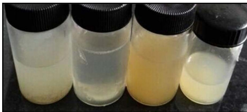
Figure 5. Appearance pictures of HMLs obtained with different mass ratio of SPC and CH (From left to right ratios were 0, 2:1, 4:1, 6:1)
