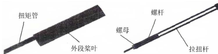
Figure 3. Changeable diameter blade shape and internal telescopic mechanism [16]
