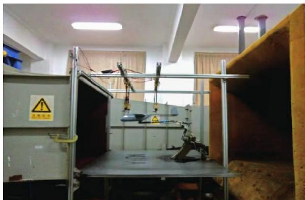
Figure 7. Hovering test table in low-speed wind tunnel [31]
