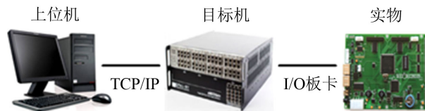
Figure 2. RT-LAB real-time system structure chart 图 2. RT-LAB 半实物仿真系统结构图
