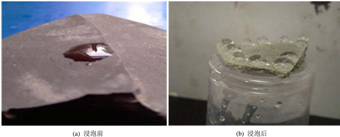
Figure 3. The effect of amino alcohol on surface hydrophilicity of rocks 图 3. 胺基硅醇对岩石表面亲水性影响
