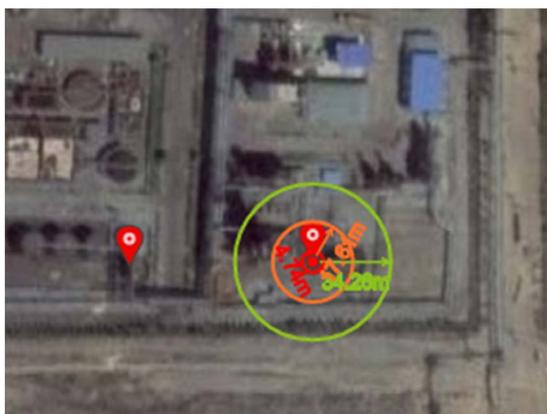
**Figure 4.** Simulation range of vapor cloud explosion damage in crude benzene intermediate storage tank
