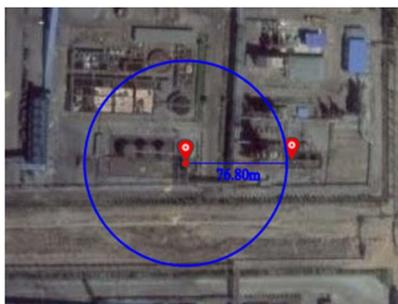
**Figure 10.** Risk-based external safety protection distance map for crude benzene storage tank (personal risk value  $3 \times 10^{-6}$ )
