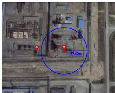
**Figure 11.** Risk-based external safety protection distance map for crude benzene intermediate storage tank (personal risk value  $3 \times 10^{-6}$ )
