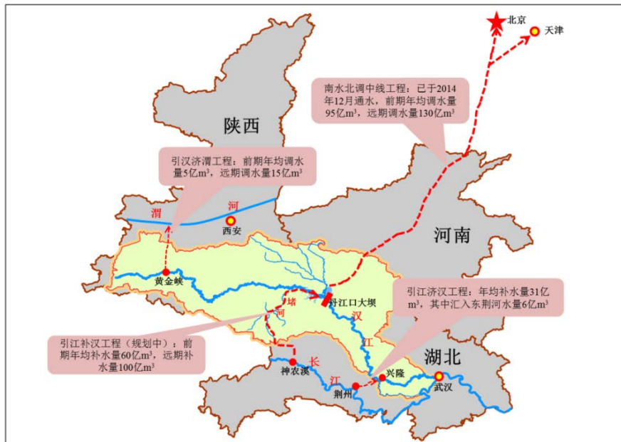
Figure 4. The trans-valley water diversion projects relate to Hanjiang River basin 图 4. 汉江流域跨流域调水示意图
