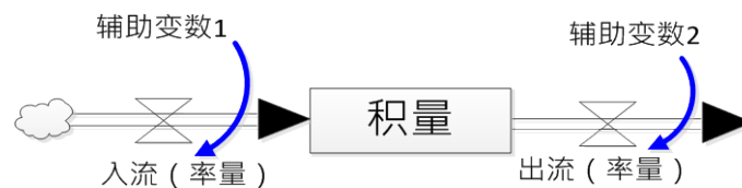
Figure 4. Architecture of system dynamic model
