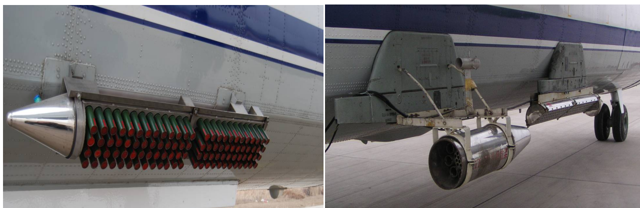
Figure 2. Airborne flame bomb and flame tube launching devices 图 2. 机载焰弹发射和焰条播撒装置
