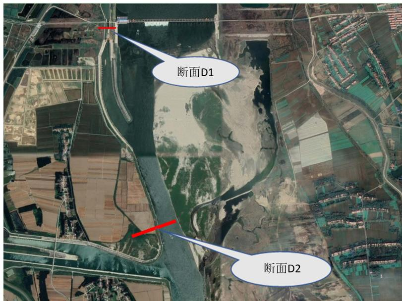
Figure 1. Schematic diagram of the layout of the hydrological test section under the dam of the Xinglong water control project
