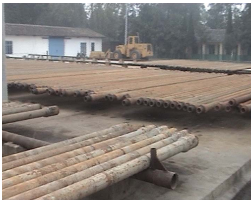
Figure 2. The stacking condition of in-service field drilling pipes
