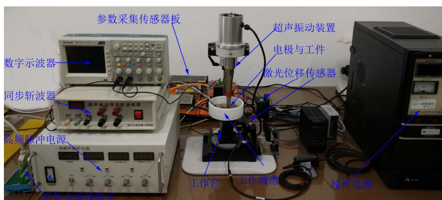
Figure 8. Ultrasonic compound electric machining system diagram 图 8. 超声复合电加工系统图
