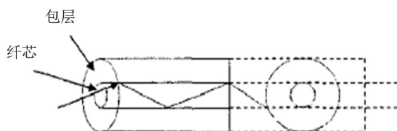
Figure 2. The basic structure of optical fiber
