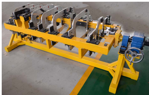
Figure 6. Typical flexible fuselage assembly tooling structure of UAV
