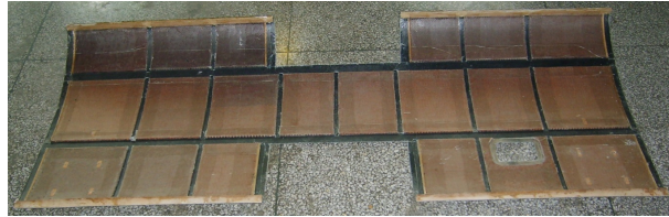
Figure 2. Typical wing skin structure of UAV 图 2. 无人机机翼壁板典型结构
