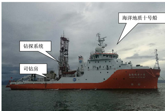
Figure 1. Marine geology ship 10 has installed a shipborne drilling system
