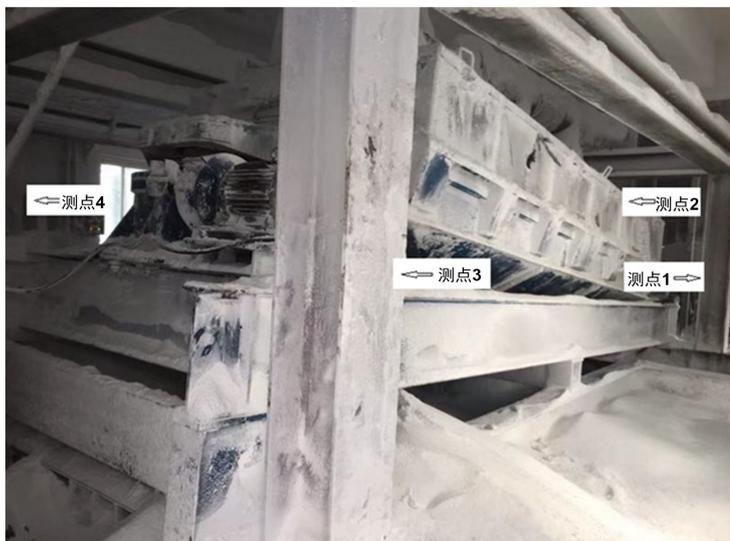
**Figure 1.** Layout of the measuring points in the urea packaging building
